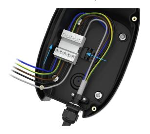
8 For dynamic load balancing, insert wires into the small connector
